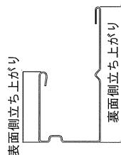
目地部材A 断面図(例) (Example cross-section diagram of Type A base material)
