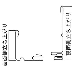
目地部材B 断面図(例) (Example cross-section diagram of Type B base material)
